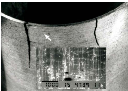
HEAT CHECK CRACKING
